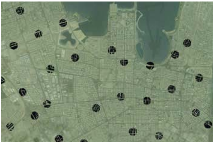
Figure 1: Halton sequence of coordinates used for sampling locales win an urban area
